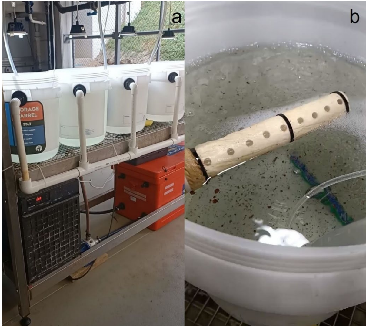
Figure 9. (a) A simple recirculating system with four 30 L vessels, downwelling lights ( 50 \mu\text{mol m}^{-2} \text{s}^{-1} ), thermally regulated water ( 19^\circ\text{C} ) and adequate nutrient supply ( 0.1 \text{ g L}^{-1} Cell-Hi ® ); (b) tetrasporophyte fragments inoculating the culture.
